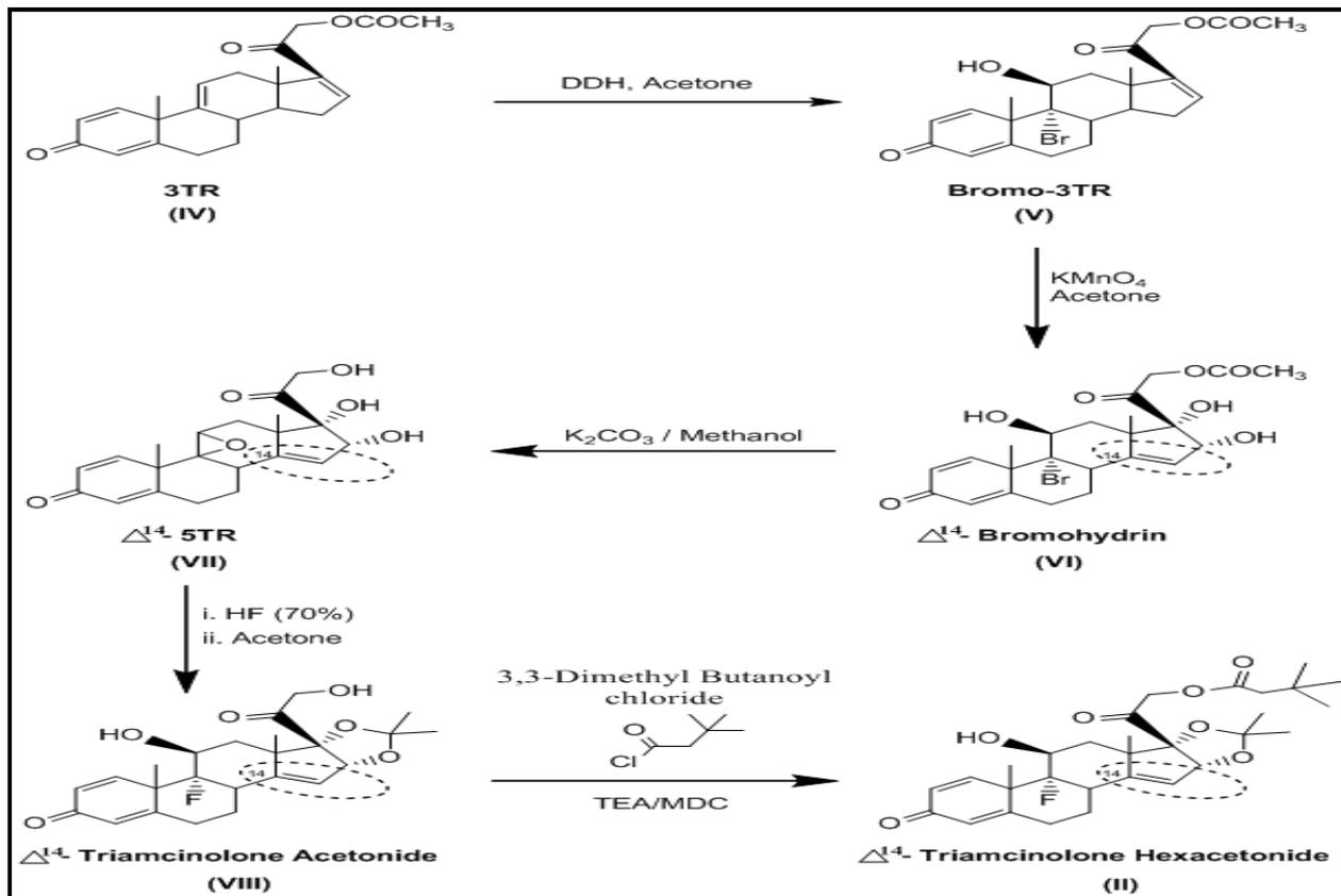
Figure No.1: Reaction Scheme: Route of synthesis of  $\Delta^{14}$ -Triamcinolone Hexaacetonide
